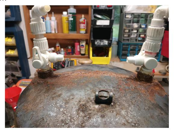
Install the valves on the new tank using Teflon tape on top of pipe dope.
